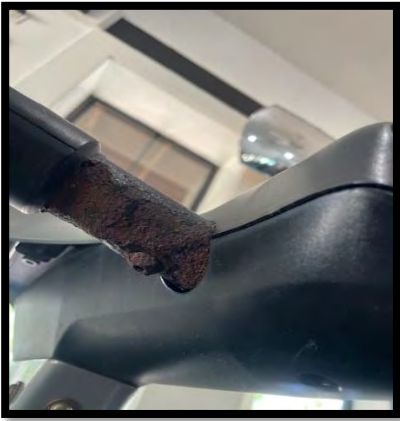
Addressed some rust on treadmill crossbar
