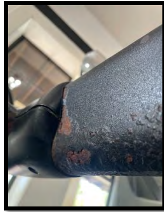
Addressed some rust on treadmill crossbar
